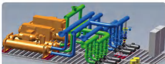
04 户内撬块装配式 Indoor pry block assembly type
